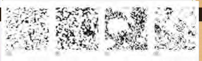
(a) Fontainebleau sandstone ( \Phi=13\% , a = 5.7 \text{ m} ), (b) Berea sandstone ( \Phi= 29\% , a = 4.4 \text{ m} ), (c) a dual scale reservoir sandstone ( \Phi = 24\% , a=2.6 \text{ m} ), and (d) a multiscale carbonate rock ( \Phi = 14\% , a=1.1 \text{ m} ). Here notes porosity, and a the voxel size.
